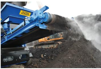
1200mm wide 2.3m high fines stockpile belt, to ensure smooth fines collection and stockpiling
