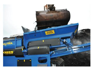
3.5 Cubic Tonne variable speed Feed Hopper, spill plates optional
