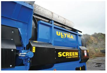
High wear brush to clean the trommel drum mesh, ensuring maximum output
